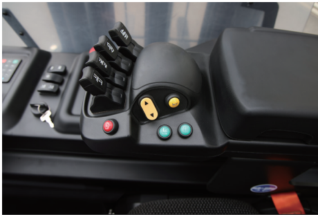
Centralized control console with fingertip operation.
