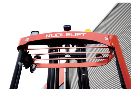
LED lighting and safety blue lights.
