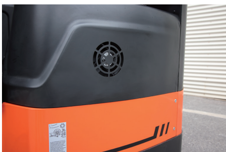
Motor cooling system.
