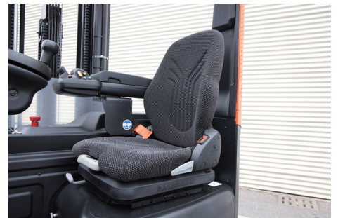
(Grammer) Suspension seat with high-elastic shock absorption.
