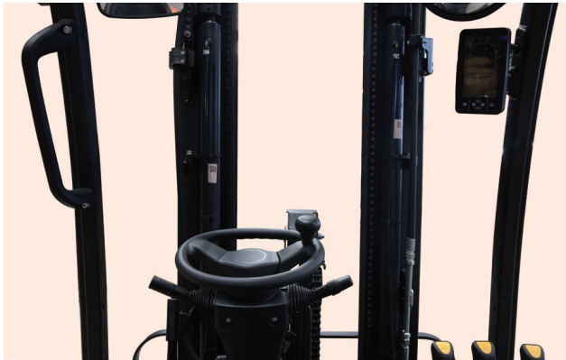
The wide-view mast makes handling cargo more convenient.
