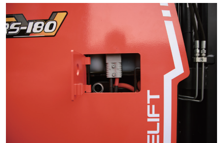
Battery charging port
