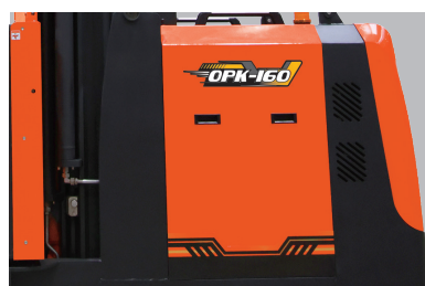
Side-accessible battery (can be used on either side)
