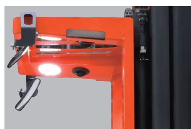
LED work lights and fan
