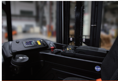
Centralized fingertip control console
