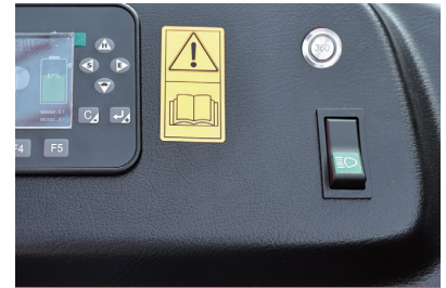
Real-time switching between 180° and 360° steering modes
